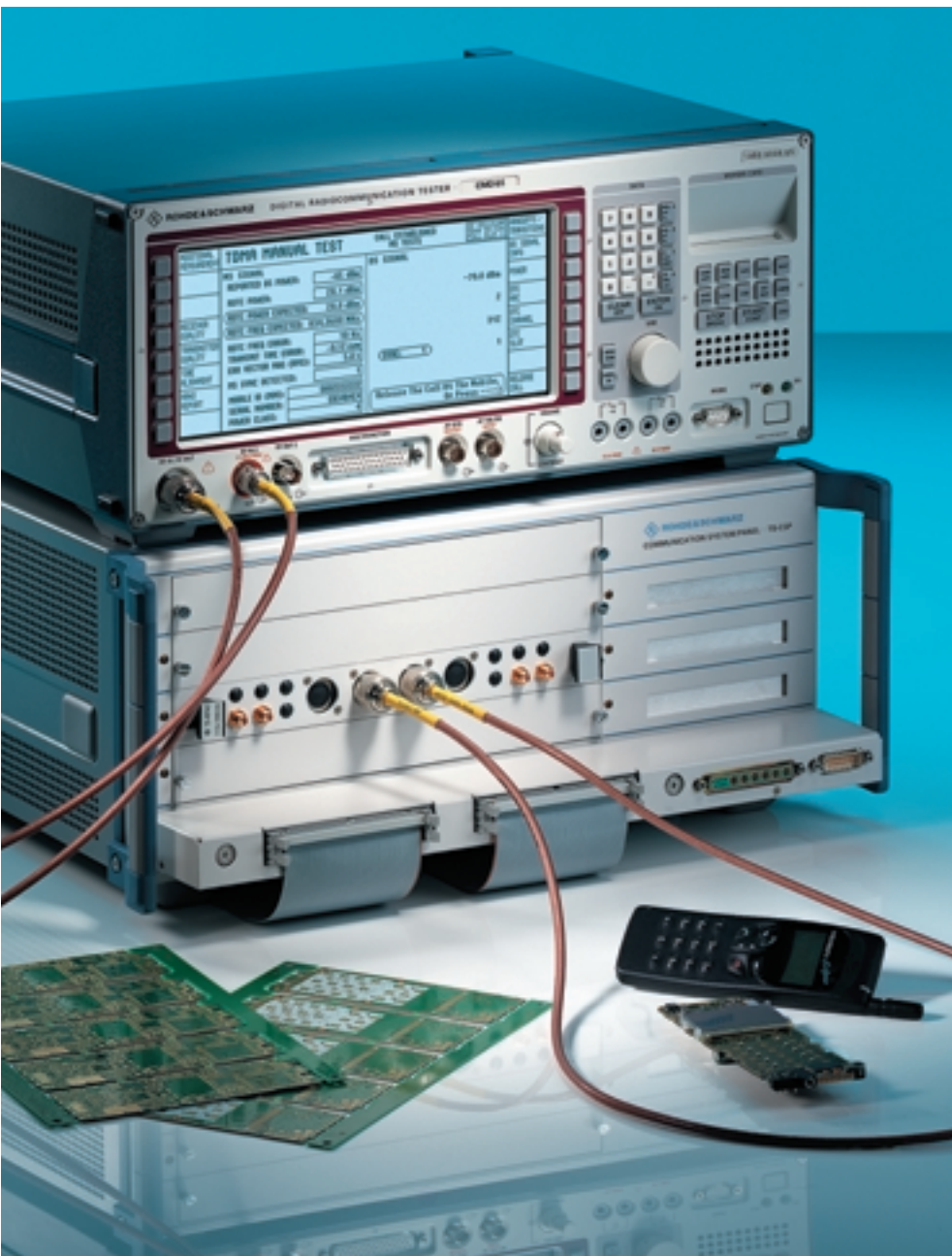
FIG 1 Communication System Panel TS-CSP – switching center for test systems (here in conjunction with Digital Radiocommunication Tester CMD 65 for testing mobile phones)
