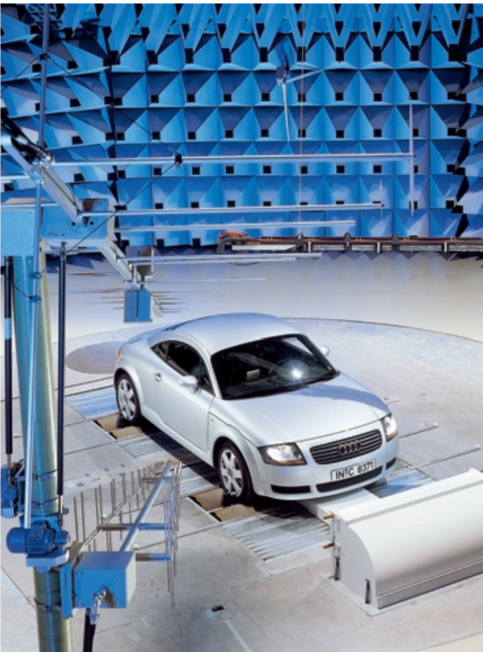
FIG 1 Measurements are performed automatically in the large anechoic chamber, so the operator can fully concentrate on EUT response
